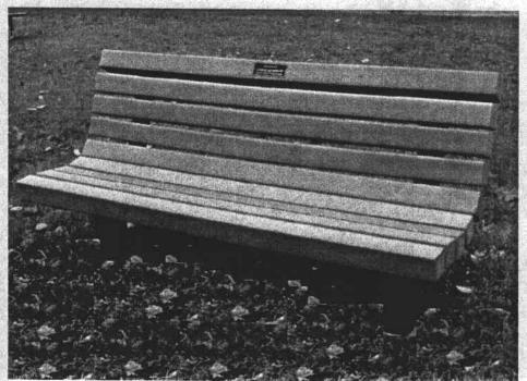
The contoured supports are  $3/8" \times 4"$  rolled steel, shaped to provide a smooth, comfortable seat and backrest. The legs are 2-  $\frac{1}{2}"$  square steel support tubing, welded to an arched  $3/8" \times 4"$  formed steel base. The frame is coated black for durability and an attractive appearance. The slats are  $4" \times 4"$  cedar-color recycled plastic. The bench is mounted directly into the ground, and each leg is anchored with concrete.
