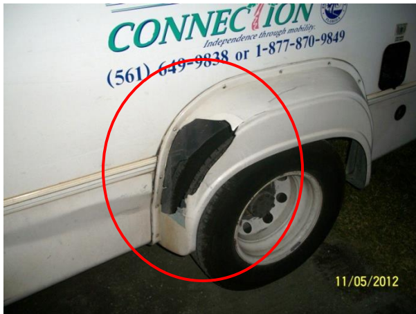
Severe fender damage
