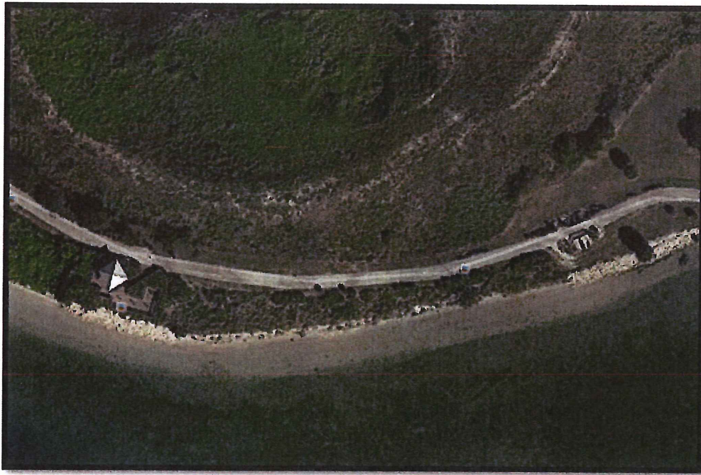
Southwest corner of Peanut Island is experiencing severe erosion Project includes armoring 375 L.F. of shoreline with rip rap
