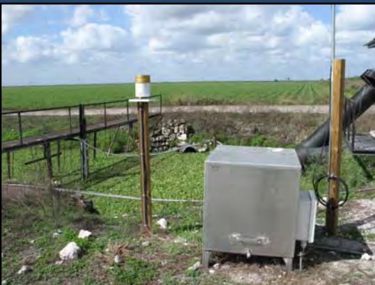
Rain gauge, ½ to 1-inch rainfall detention
