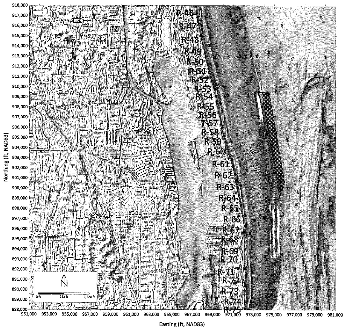
Figure 1 – Recent bathymetry at Singer Island, showing the rough seabed in the nearshore between R060 and R067.
