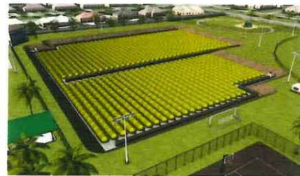
Design Image of StormTech Chambers (above) Athletic Sports Field (below)
