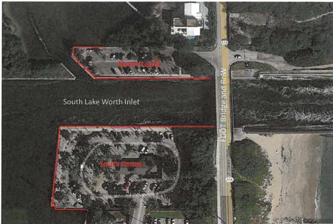
Figure 1. Location Map. Seawalls to be replaced are shown in red. Base map from Google Earth.
