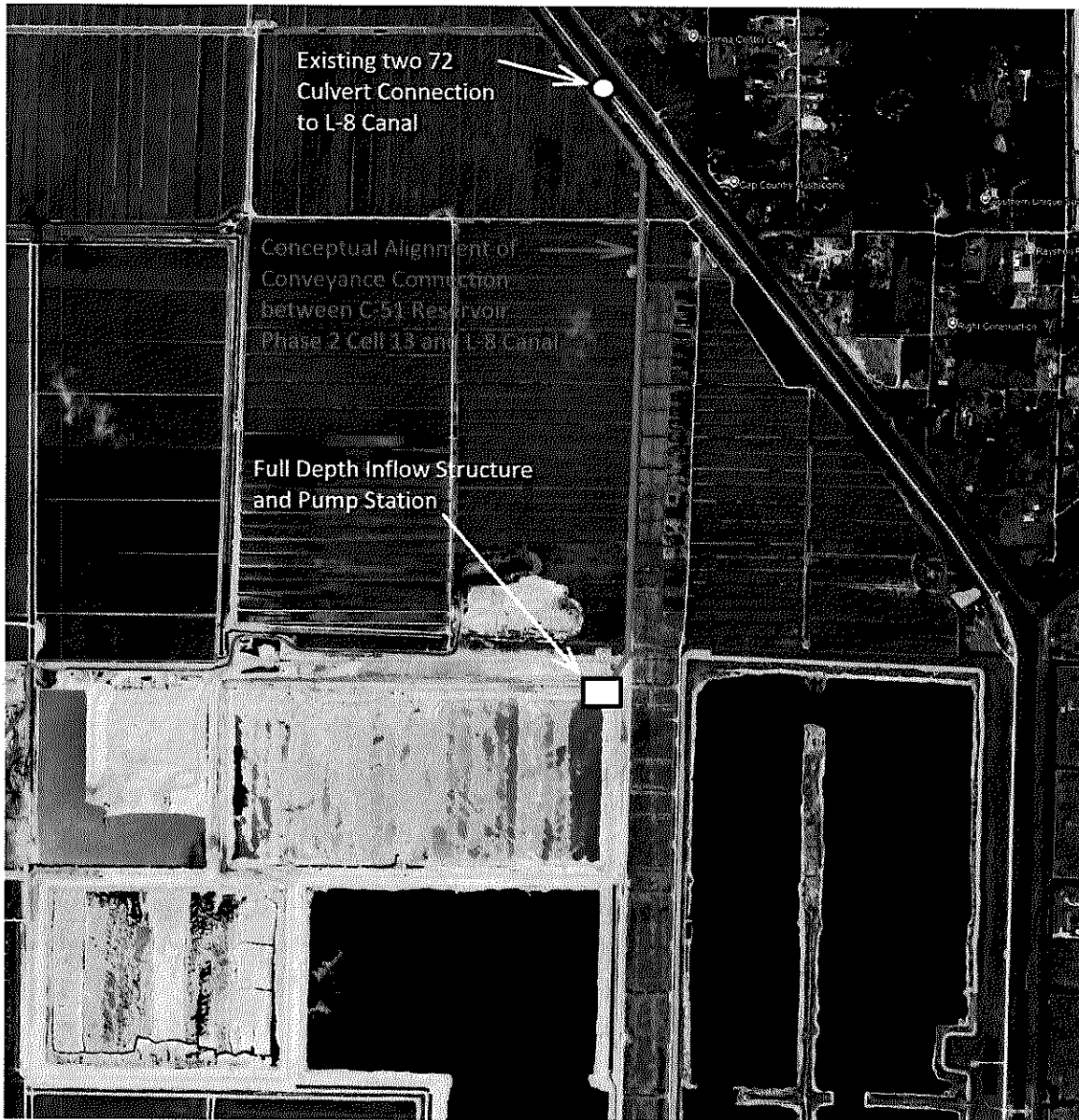
Figure 3. C-51 Reservoir Project Features Map
