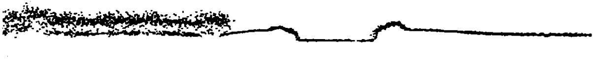
Figure 3. This is the vertical profile of a transect from crop canopy to harvested (from left to right). There are many second returns (in red). In the middle is the ditch (water filled). Either side has the elevated dykes. Note that there are practically no second returns from the bare soil (only first returns).
