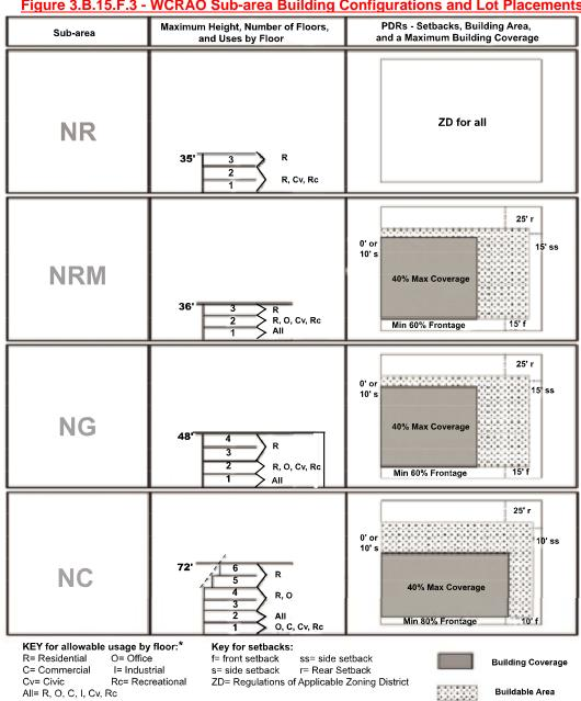
Figure 3.B.15.F.3 - WCRAO Sub-area Building Configurations and Lot Placements
