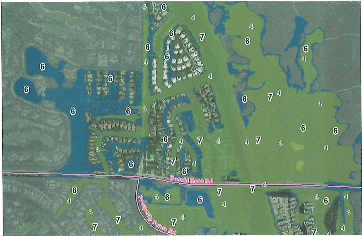
Figure 1 - Proposed Base Floor Elevation in Larger Font (Existing Base Floor Elevation in Small Font)
