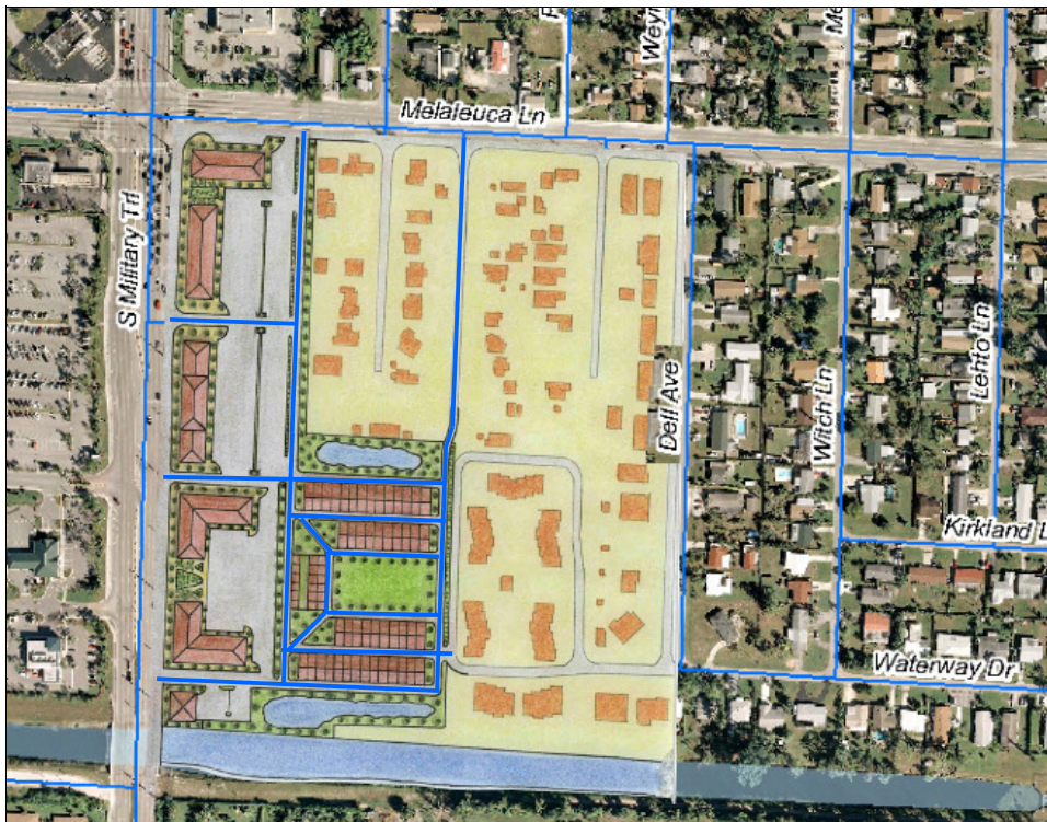
This illustration, showing both the existing development and proposed redevelopment, depicts how narrow depth infill parcels along commercial corridors can be retrofitted to provide parallel alternate vehicular routes, thereby reducing potential trips on arterial roadways.
