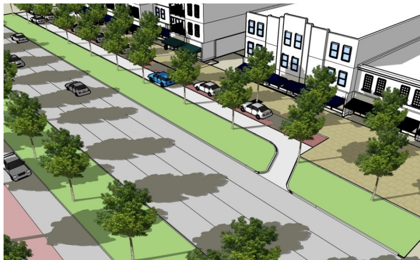
47 FIGURE 3.B.17.F – TYPICAL EXAMPLE OF SLIP STREET FRONTAGE
